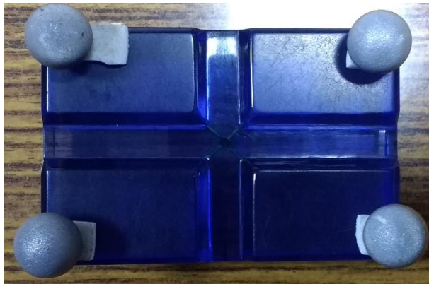
Fig. 7 The rigid body used for experimentation (It is ideal to have number of markers = Number of vertices of top face so as to avoid IR reflection amongst the markers and to ensure proper detection of the body)
