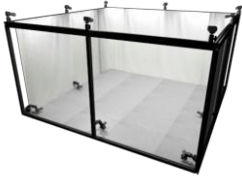
Fig. 25 separation of capture volume using translucent curtains
