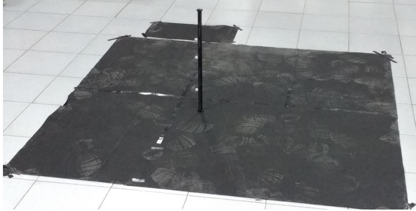
Fig. 6 Set-up for Point objects on a Dark surface with Bright lighting in 3D
