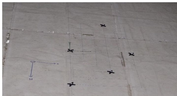
Fig. 5. Set-up for Point objects on a reflective Surface with Bright lighting in 2D
